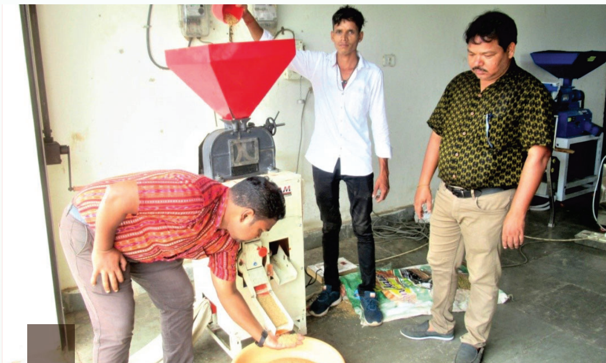
Load Test of Rubber Roll Sheller Cum Polisher of Sree Ram Udyog
