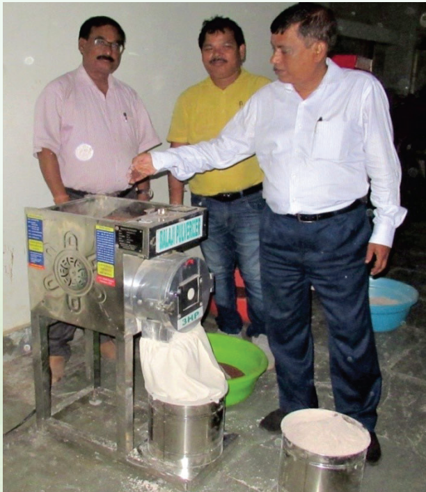
Load Test of Pulverizer of Punjab Machinery Works, Raipur
