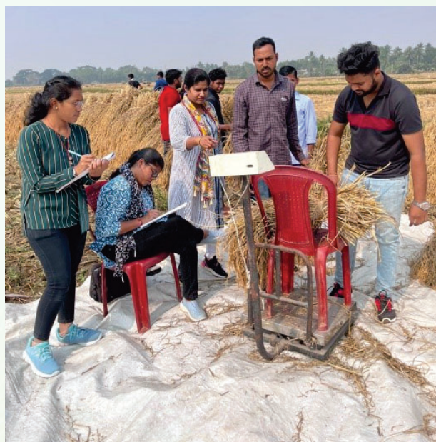
Measurement of straw bale for load testing of axial flow paddy thresher at Tarapur Jagatsinghpur
