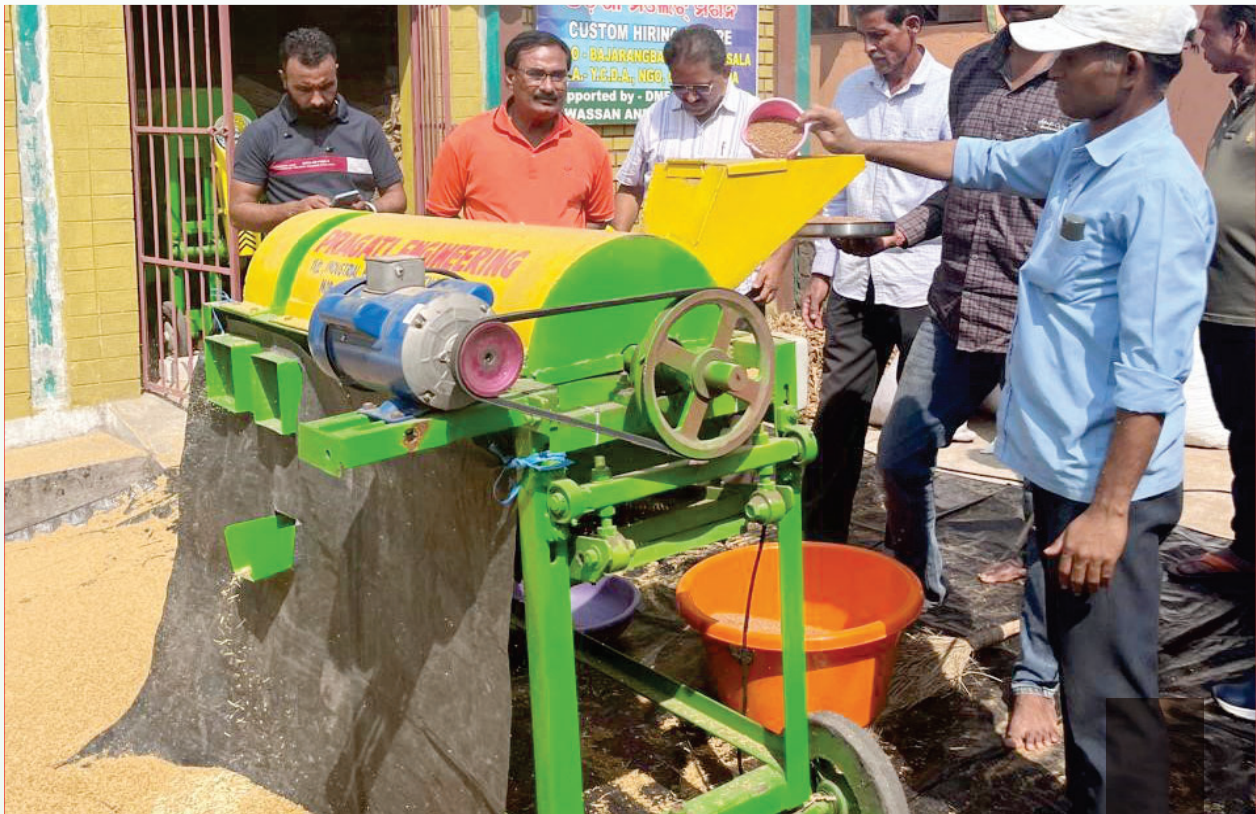
Testing of Millet Thresher cum Pearler by the Engineers of SLFMTTC in presence of manufacturer at Chhendipada, Anugul
