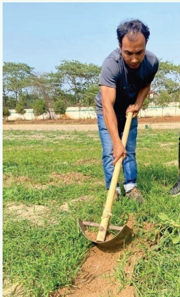
Testing of Curve Weeder with U-Shaped Design at SLFMTTC Innovated by an Innovator from West Bengal
