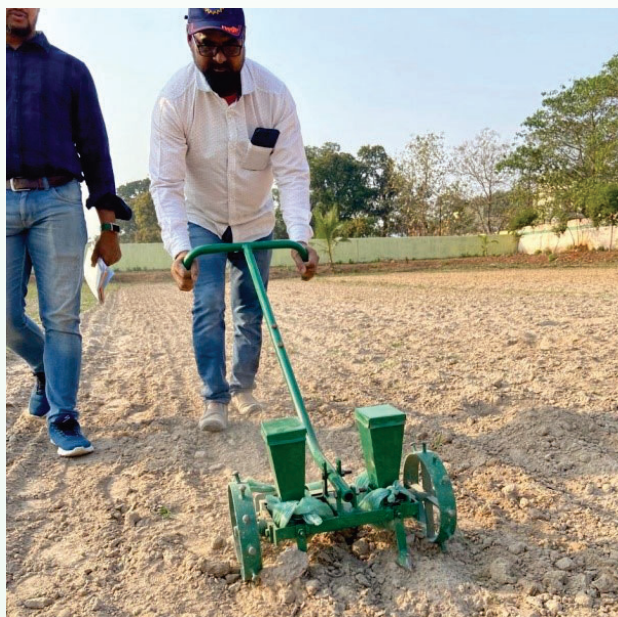
Testing of Jute Seed dibbler, a specialized agricultural tool at SLFMTTC developed by an Innovator from West Bengal
