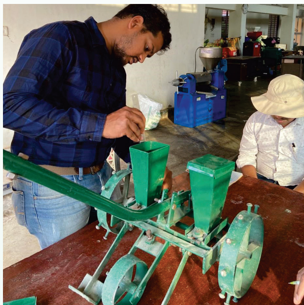
Testing of Jute Seed dibbler, a specialized agricultural tool at SLFMTTC developed by an Innovator from West Bengal
