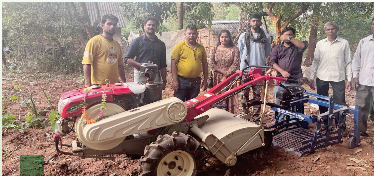
Performance Testing of Potato Digger by Testing Engineers of SLFMTTC along with NIF Team and Innovator at Raikia, Kandhamal, Odisha
