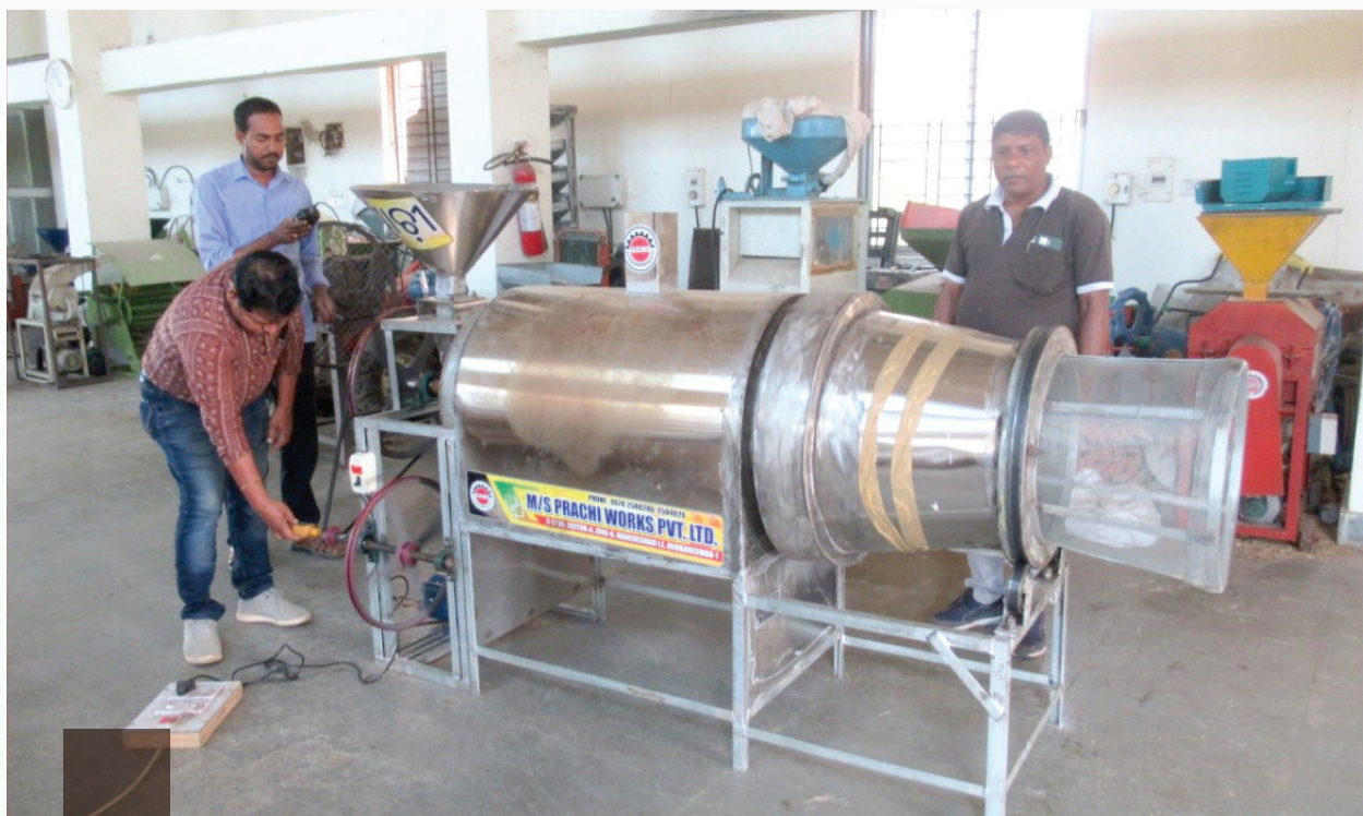
No Load Test of Rice Puffing Machine of M/S Prachi Works Bhubaneswar
