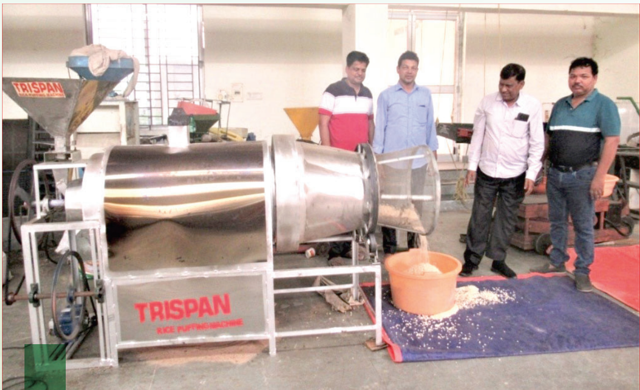
Load Test of Rice Puffing Machine of Trispan Farm Equipment and Engineering, Jagatsinghpur
