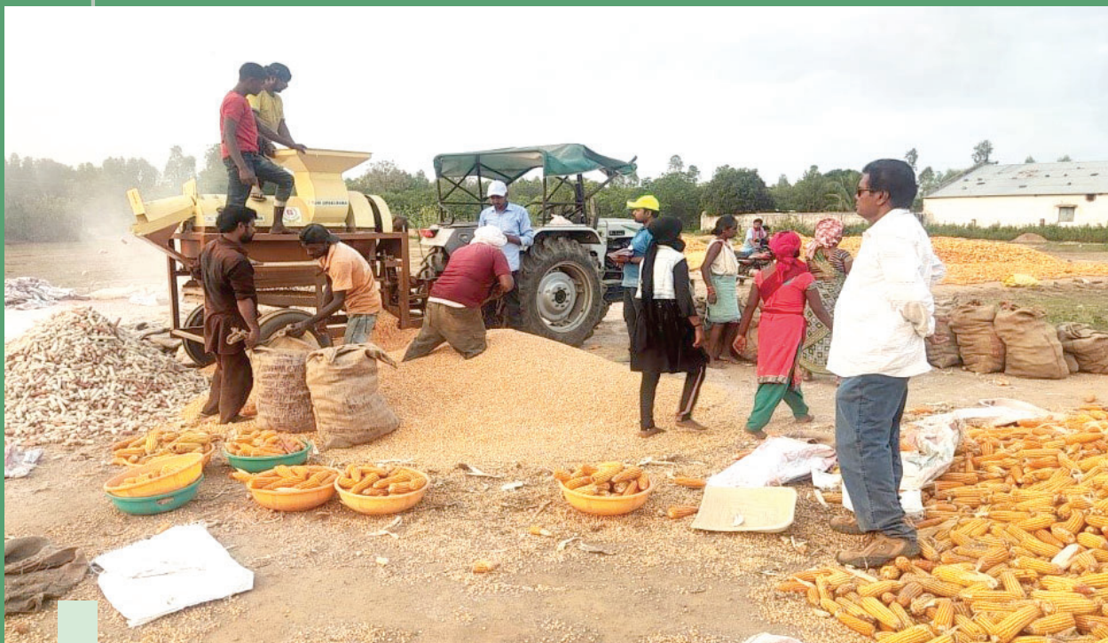
Testing of Tractor operated Maize Thresher by Testing Engineer of SLFMTTC at Umerkote, Nabrangpur
